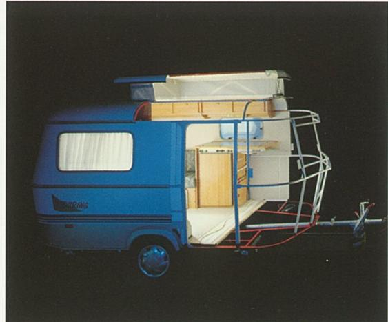
The tubular steel frame structure making up the skeleton of an Eriba Touring caravan was developed over 45 years ago, and has not been superseded as a perfect element for making a strong, rigid, durable, lightweight caravan in superbly aerodynamic design.
